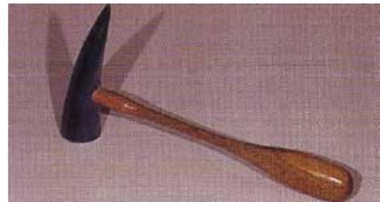
the horn is well clamped before beginning to drill the hole in the horn for the handle. My handle was tapered from 1/2" to 3/8" diameter so I drilled a 3/8" diameter hole through the horn. I then used a tapered reamer to taper the hole in the horn from 1/2" to 3/8" diameter. The drill size you will use depends on the smallest diameter of the handle you purchase.
