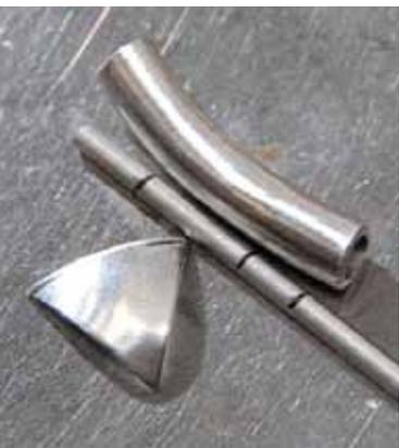
Lining up smaller tubing to create hinges.
