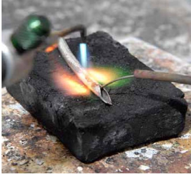
Benefit from capillary action while soldering the seam of hand-made tubing.
